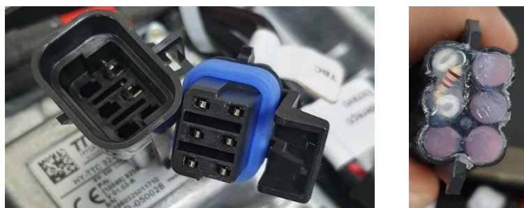
Fig. 6.30: Conexões TBC (Threaded Bottom Connection).
